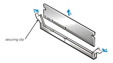
Figure 8-7. Removing a Memory Module
